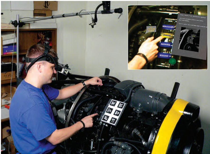
An augmented-reality application developed at Columbia University. The “opportunistic controls” shown in this image are virtual buttons on a raised portion of an aircraft engine housing, providing haptic feedback for a maintenance technician.
