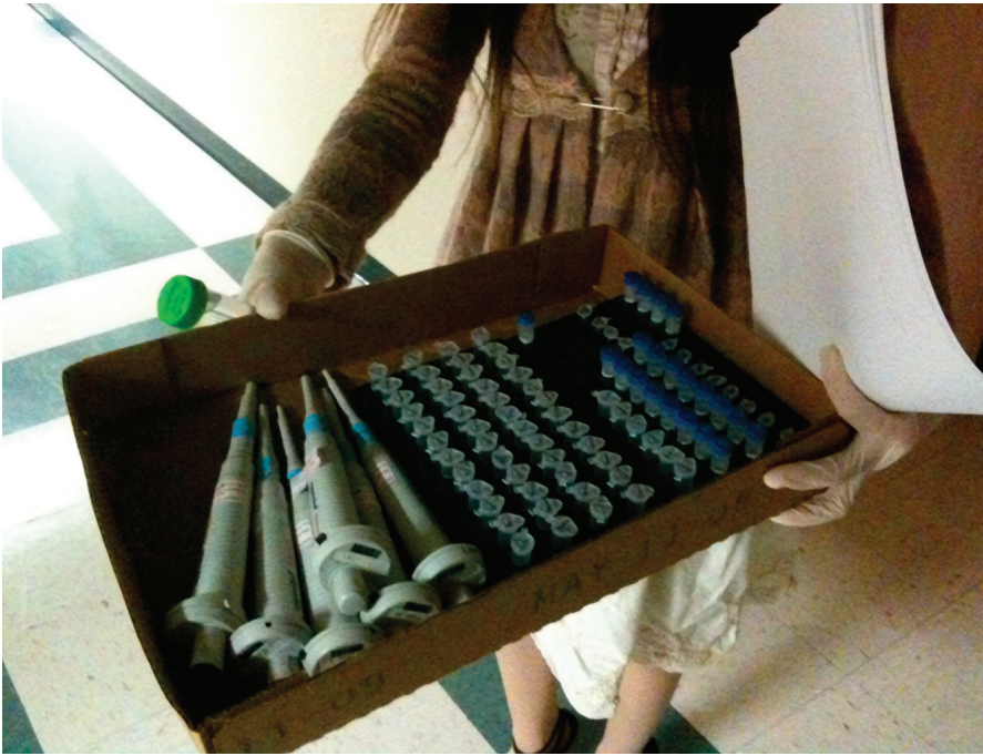
Heading to the instrument room at Caltech. In the box are the pipettes and test tubes containing molecules for a biochemical circuit: the 74 tubes each contain one type of DNA logic gate or fuel, and the eight tubes contain input signal strands. To get the DNA circuit running, the 74 gate and fuel molecules must be mixed to form the functional circuit, and a combination of the eight input signal strands must be added. Fluorescence must then be monitored during the next 10 hours to determine the circuit's output.
